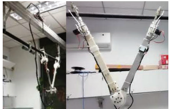
Fig. 5. The inspection bionic-robot platform.
