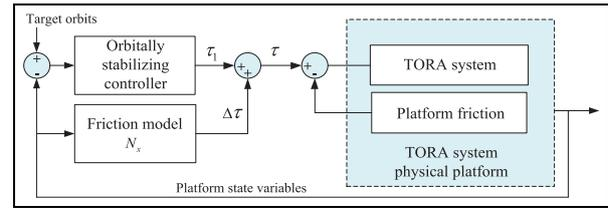
Figure 4. The redesign process of the orbitally stabilizing controller with compensation control.
