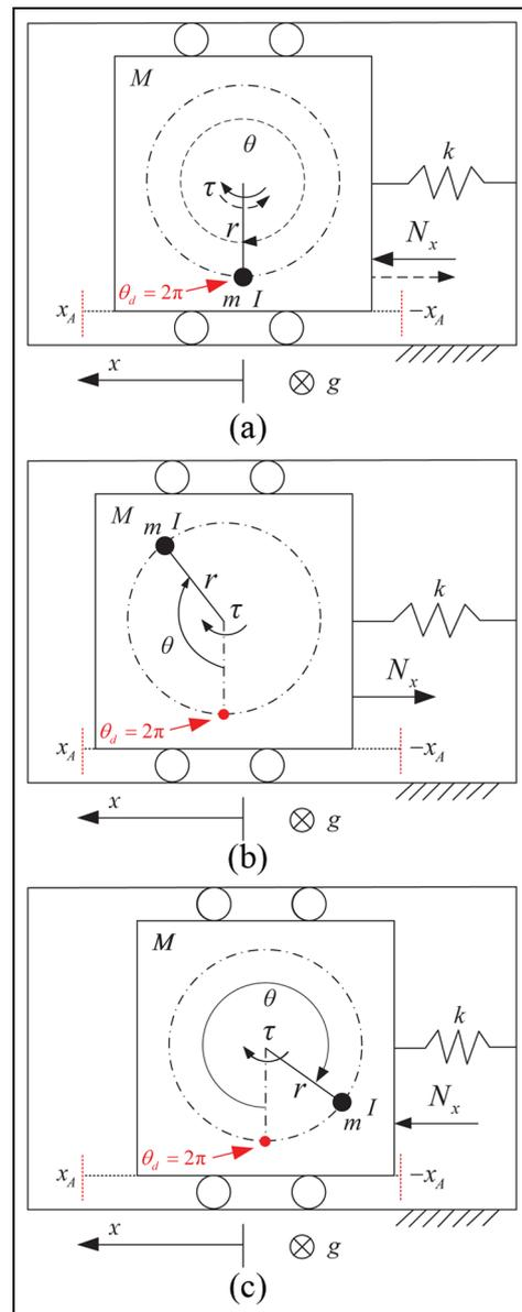
**Figure 2.** The tracking process of orbitally stabilizing control for TORA system from equilibrium point to the target orbits:  $x_d(t) = x_A \sin((2\pi/T)t + \varphi)$ ,  $\theta_d = 2\pi$ . (a) initial condition; (b) condition of  $0 < \theta < \pi$ ; (c) condition of  $\pi < \theta < 2 * \pi$ .
