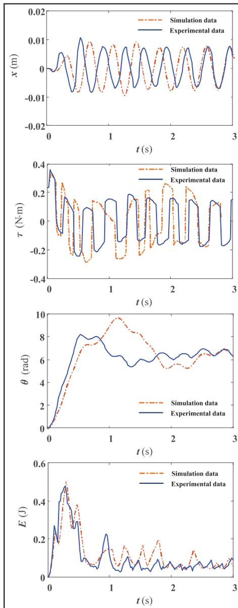
**Figure 8.** Experimental results of the physical control input torque  $\tau$  on TORA platform; target orbits are chosen as  $x_d(t) = 0.008 \sin(16.11t - 0.65\pi)$ ,  $\theta_d = 2\pi$ .
