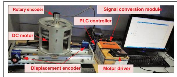
**Figure 7.** The outline of TORA system platform.
