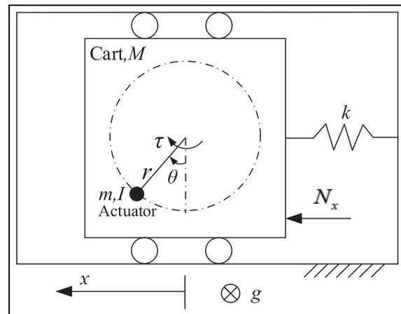
Figure 1. TORA system configuration.
