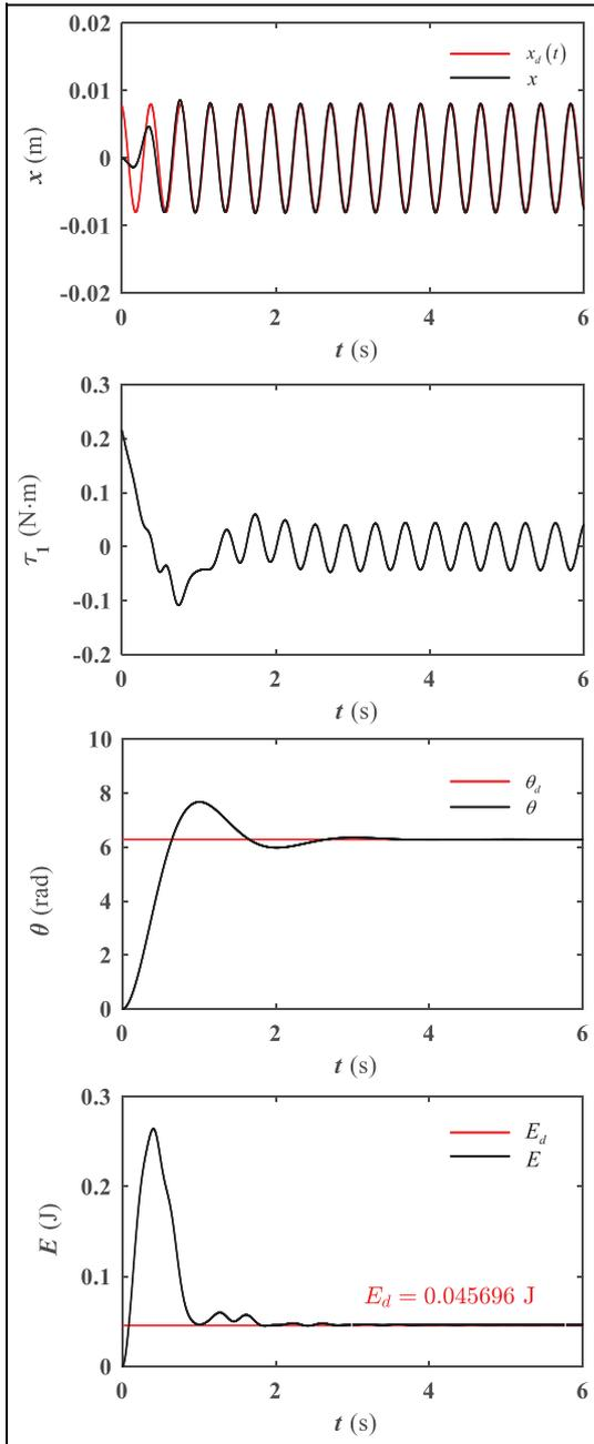
**Figure 3.** Simulation results of the proposed controller  $\tau_1$  for TORA system and the target orbits are chosen as  $x_d(t) = 0.008 \sin(16.11t + 0.57\pi)$ ,  $\theta_d = 2\pi$ .
