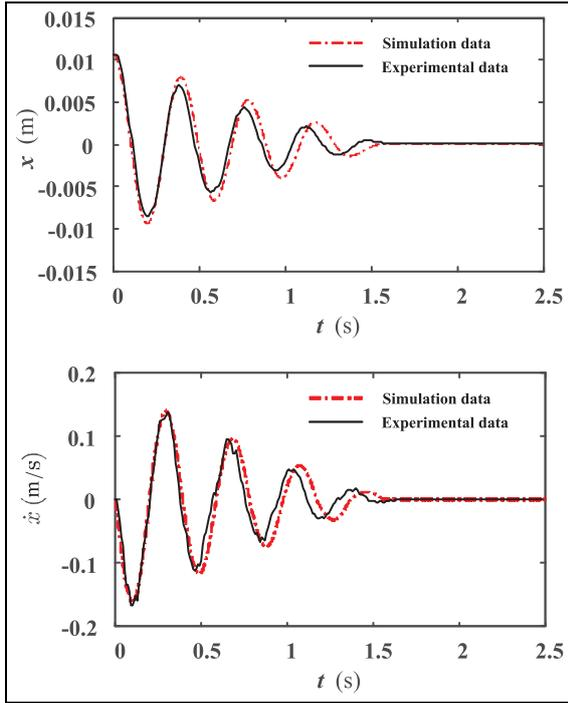
**Figure 5.** The position and velocity of the translational cart in free oscillation; initial TORA conditions are chosen as  $[x, \dot{x}, \theta, \dot{\theta}, \tau]^T|_{(t=0)} = [0.0107, 0, \pi/2, 0, 0]^T$  (black solid line: experimental data based on TORA platform; red dashed line: simulation data based on TORA dynamics).
